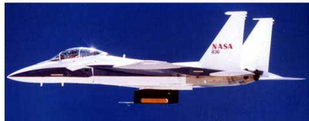
Figure 12: Boundary Layer Heating Experiment in Flight
